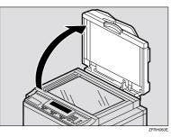
**2** Place the original face down on the exposure glass. The original should be aligned to the rear left corner.
